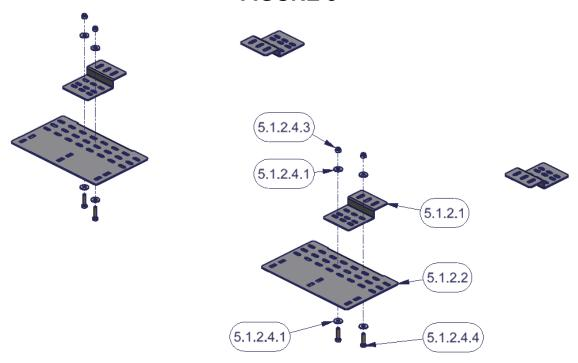
6. Fasten the assembled brackets to the bottom of the drawer enclosure with the hardware illustrated. Be sure they are oriented and located as shown for a standard installation. (See Figure 4)
