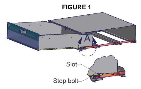
4. For a standard mounting application as described above fasten only (1) #8 mounting bracket to the drawer enclosure with the illustrated hardware. These bolts are difficult to reach; Use a ½" shallow socket with a long extension and a ratchet (Universal joint also helps) and a ½" wrench on the other end. Unbolting the slide using a 7/16" wrench will make things easier as well. **These parts and fasteners are included with the drawer.** (See Figure 2)
