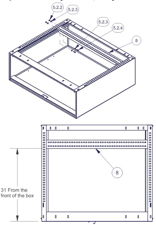
5. Assemble the mounting brackets as illustrated. Be sure left and right sides are assembled opposite. (See Figure 3) (NOTE: If your drawer is narrower than 24", both of the #5.1.2.2 support plates will not fit. These plates were designed to give additional support for wider drawers so they are not necessary on narrow drawers. The assembled riser brackets can be bolted directly to the #8 adjustable mounting brackets included with the drawer or you can use one plate if needed.)
