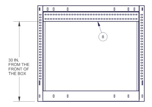
2. Assemble the mounting brackets as illustrated. Be sure left and right sides are assembled opposite. (See Figure 3)
