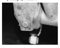
5. Securely fasten the stock bolt removed in step 1 into its original position.
