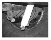
6. Connect the shock to the bracket extension using the new bolt included with the kit.
