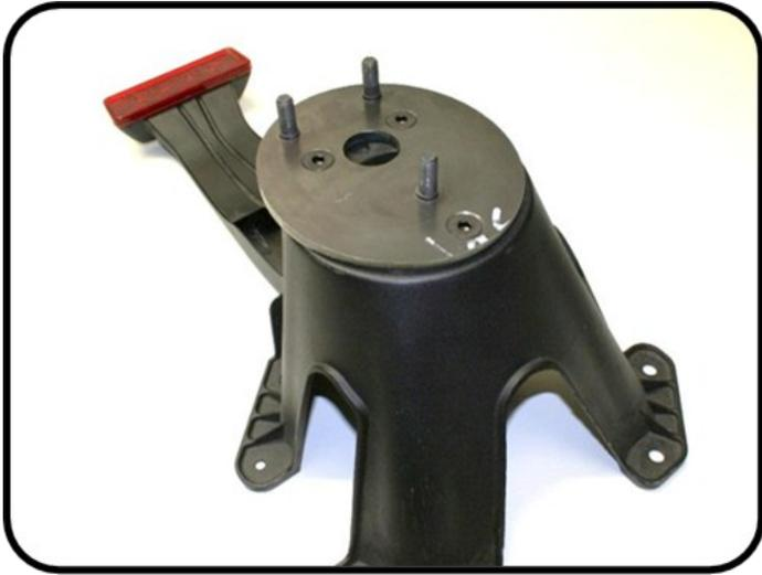
8. Install the three socket head bolts through the plate. One will thread into the factory lower hole. Fasten the other two by using the supplied Stover lock nuts.
