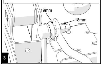
Install the swivel end of the link into the sway bar from the outside. Install the new lock nut using the 19mm end wrench and the 6mm allen wrench. Torque to 66 ft-lbs
