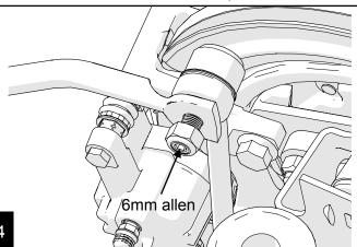
Using the 18mm install the factory hardware and two provided washers on the lower end of the link. Place the washers on either side of the bushing. Torque to 75 ft-lbs.
