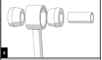
Install the lower end of the new link on the sway bar. Torque to 40 ft-lbs.
