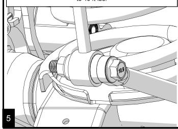
Install the upper end of the new link onto the frame. Torque to 40 ft-lbs. Repeat on other side.
