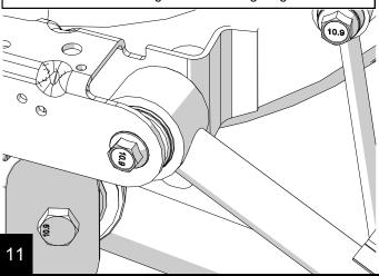
Install the flex-joint end of the arm into the axle side bracket with the original hardware. Tighten the nut and bolt finger tight. Reinstall the parking brake cable/bracket and ABS wiring. Before final tightening, lower the vehicle. Torque both nuts to 55 ft-lbs.
