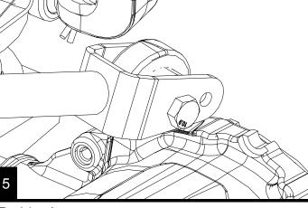
Install the frame side nut and bolt. If you are only installing the upper arms, tighten finger tight. Lower the vehicle and torque both bolts to 60 ft-lbs, Otherwise, install lower arms before lowering the vehicle.
