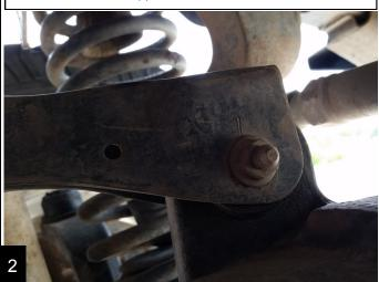
Remove the upper frame side bolt with an 18mm. The nut is a flag nut. Remove arm.
