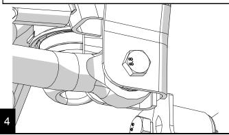
Install the track bar into the axle bracket. Tighten finger tight. With the vehicle on the ground, torque both bolts to 125 ft-lbs.
