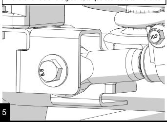
To center the axle under the Jeep, use a 15mm to loosen the adjustment sleeve clamps and turn the sleeve. When adjustment is finalized, torque clamp bolts to 45 ft-lbs.
