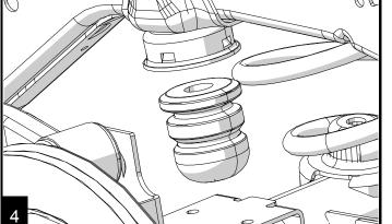
Apply grease to the bumpstop and the extension. Or just the strike pad.
