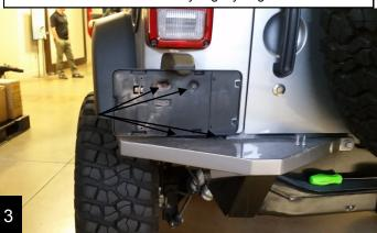
Unclip the wiring harness from the inside of the bracket by pulling up on the tab shown and pulling the harness out.
