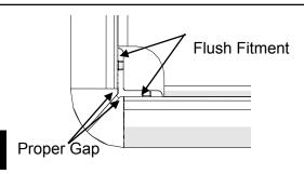
Install top aluminum rails with (8) # 332 bolts and (8) #651390 T-nuts. The 1/16" corner gap should be similar to step 10. Torque to 5 FT-LBS (7 Nm).
