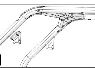
The rack is adjustable both vertically as well as front to back. Slide the rack forward until there is a 1/4" gap between the rack and back seat. Torque the bolts to 5 FT-LBS (7 Nm).
