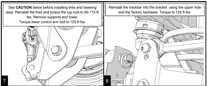
**Caution:** The trackbar bolt can rub on the rear driver side spring. To avoid this turn/clock the rear springs to where the pigtail end is to the rear of the Jeep.
