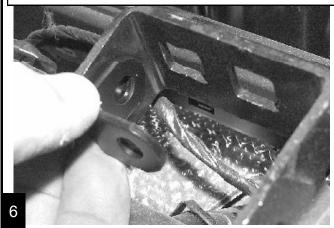
Take the end of the cable and run it through the top of the thumb lever down through the shift boot then through the center console.
