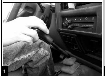
You want to slide the rubber bushing over the shift lever for a tight fit. (You might need to ream the bushing out with a drill to fit over your shift lever, but do not remove too much material, or you won't get a tight fit.)
