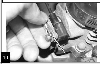
After installation, check the operation of the accelerator pedal and the hand throttle. Do this with the emergency brake on and the transmission in neutral, so as to avoid injury.
