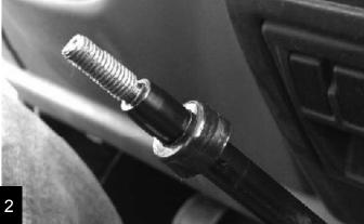
Attach the thumb lever to the rubber bushing,
