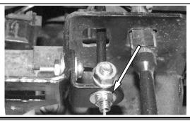
Mount the cable to the throttle linkage by wrapping the cable around the pin and then crimp the cable with the aluminum quick clamp. The "8" clip is then used to retain the cable.
