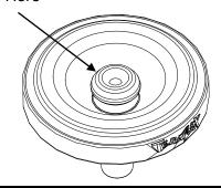
Install the spring. Raise the axle high enough to reinstall the shocks. Torque shock bolts to 56 ft-lbs (76 Nm).
