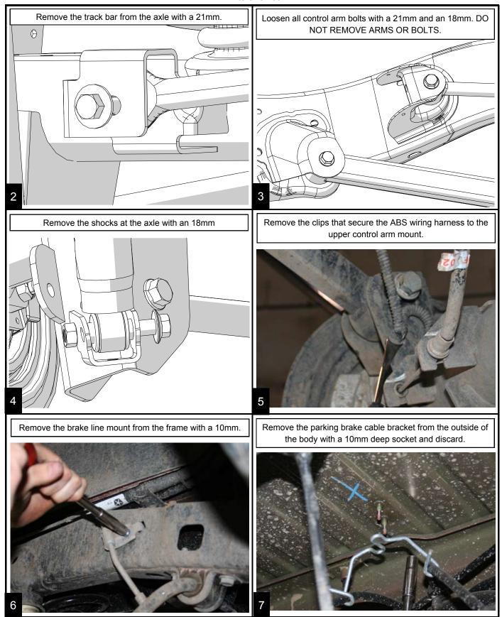
Lower the axle and remove the springs. Do not over stretch the ABS, breather and brake lines. Some kits may require disconnecting the rear sway bar links.
