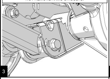
Disconnect the shocks at the axle with an 18mm.
