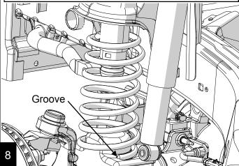
Reconnect the shocks with an 18mm. Torque to 56 ft-lbs (76 Nm). If installing on a lift, proceed to rear step 1 and install the rear spacers.
