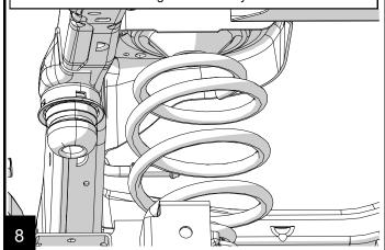
Remove the factory isolator from the upper spring perch and install onto the new spring spacer.
