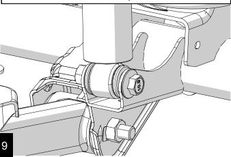
Reconnect the track bar once the vehicle is on the ground. Torque bolt to 125 ft-lbs (170 Nm) Torque wheel lug nuts to 95-115 ft-lbs (129-155 Nm).
