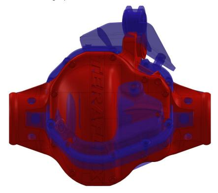
• A new ductile iron differential cover has been designed for maximum steering clearance and durability. The bottom section of the cover is nearly ¾" thick for ultimate durability when the trail gets rough. The cover features a built in "seal-breaker" to aid in cover removal for differential service.
