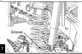
Raise the jack high enough to install the shocks. Torque to 56 ft-lbs (76 Nm). (See 999207 Shocks/Front/Installation)
