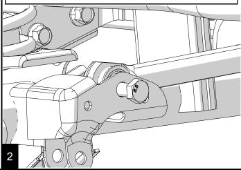
Loosen all front control arm bolts with a 21mm. DO NOT REMOVE ARMS OR BOLTS.
