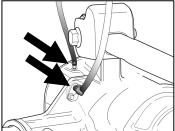
NOTE: DO NOT TIGHTEN THE CONTROL ARM BOLTS UNTIL THE JEEP IS ON THE GROUND
