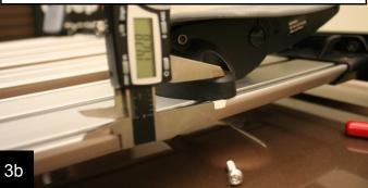
Two slats can be used to mount a cargo box. The slats will keep the box lower than using load bars, helping to reduce wind noise. This vehicle has the Thule Sonic Alpine 633s box mounted with 4 M6 x 1.0 x 30mm long stainless socket head cap screws. The Thule Xadapt 10 kit replaces the
