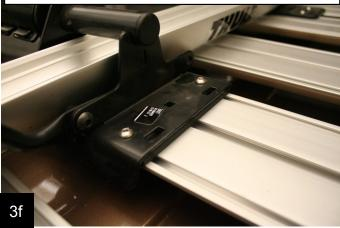
This photo shows the Thule 594XT bike rack mounted in the rear with the Thule Xadapt2 mounted between two stats for correct spacing. Two M16 x 1.0 x 12mm long stainless screws with a M6 washer are used to fasten it to the slat.
