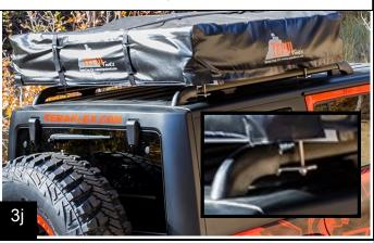
The molded in hook holes are meant to secure light loads. Do not use a ratchet strap as over tightening will cause damage.
