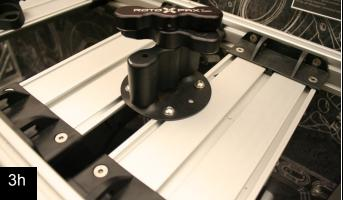
Below is a Quick Fist mount installed with a M6 x1.0 x 22mm long bolt with a washer under the head to avoid bottoming out.
