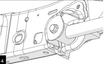
Install the adjustable end into the axle side bracket. If your vehicle has cam-bolts, either use cam-bolt eliminator washers or rotate the cam to the full forward position as shown.
