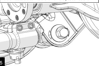
After the vehicle is on the ground and at ride height, torque the axle side bolt to 117 ft-lbs (159 Nm) and the frame side bolt to 125 ft-lbs (169 Nm). Next, gradually tighten the aluminum clamp bolts equally until a final torque of 30 ft-lbs (41 Nm) is achieved. Go back and forth between the clamp bolts a couple times to ensure proper torque.
