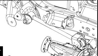
Lengthen the new Alpine arm to 18 7/8". Install the adjustable end into the frame side with the decal facing outwards. Install all bolts **finger tight**.
