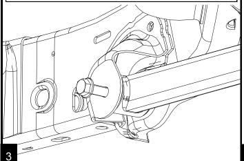
Lengthen the new Alpine arm to 23 1/8". Install the fixed end into the frame side bracket with the sticker facing outwards.
