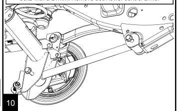
Lengthen the new Alpine arm to 20 1/8" for 2 door models and 20 1/2" for 4 door models. Torque the aluminum clamp bolts to 30 ft-lbs (41 Nm). Install the arm with the fixed end on the frame side. Install all bolts **finger tight**.
