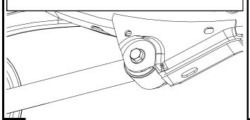
After the vehicle is on the ground, torque all bolts to 125 ft-lbs (169 Nm)
