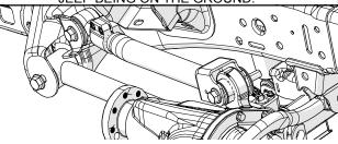
For all other kits DO NOT completely tighten any joint or bushing until the Jeep is on the ground. This is important for bushing life, flex and ride quality.
