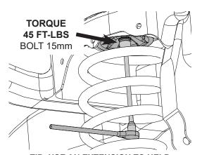
**TIP: USE AN EXTENSION TO HELP TIGHTENING / TORQUE BOLT**
