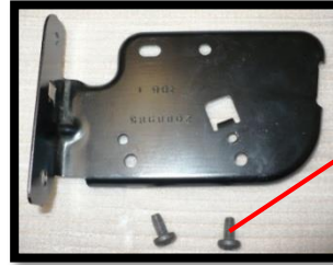
The screws are Torx T30, but if you don't have a torx bit, they remove pretty easily with a thin flathead screwdriver.
