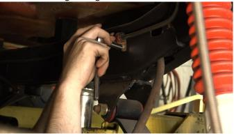
Remove any factory or aftermarket parts, linings, and/or coatings. Remove your body mount bolts and bushings from the existing crossmember.
