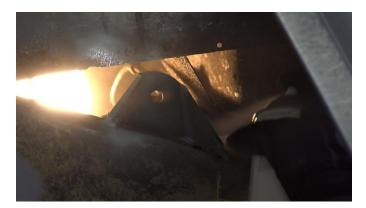
Replace the part and C-clamp and tack weld it into place to prevent it from moving later.
