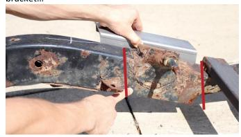
While aligning with your drawn marks of the OEM shock location.
