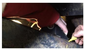
Make note of, or mark and trace, the OEM location before removal to aid in the replacement of the new part.
