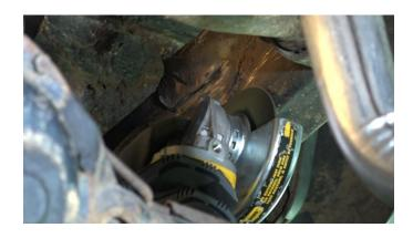
Determine and mark the weld location of the section. Place the section on the inside of the frame, as shown. Ensuring the lower angle points forward, and the rear angle avoids the shown bracket...
