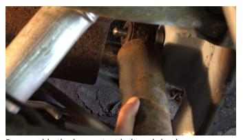
Reassemble the lower strut bolt and shock.
