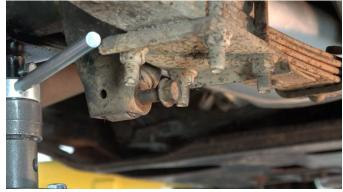
Remove the upper strut bolt connecting the shock to the Upper Rear Shock Mount and remove the shock.
