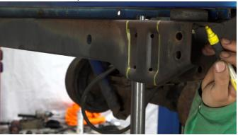
Depending on your level of experience, you may want to cut just outside of the frame rail to avoid cutting the frame. This will require you to remove any excess metal, such as welds, from the frame rails.
