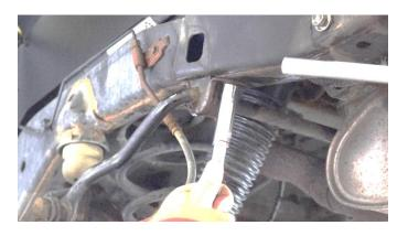
With an 18mm socket, remove the body mount bolt and bushing and set it aside to be reused later.
