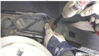
With a 22mm socket, remove the bolt securing your track bar and push it down and out of the way.
