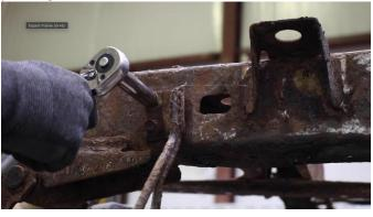
Hold the part up to the frame and take note of its coverage. Clean the frame of any rust and debris, revealing bare metal.
