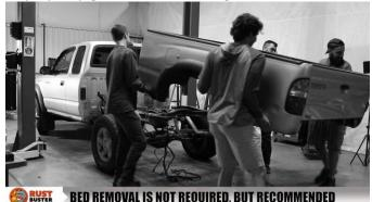
[Removing the <u>hitch and rear bumper</u> is required. Removing the bed grants complete welding access to the top most edges of the stiffeners, but it's not required]
