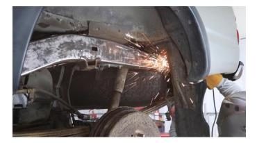
Replace the part, using existing bolt holes and body mount brackets as alignment reference points, and C-clamp it to the frame.
