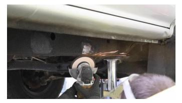
Replace the part, using the center frame hole as an alignment reference point, and C-clamp it to the frame.
