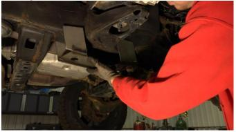
Cut away and repair any rust and debris to help prevent it transferring to the plates.
