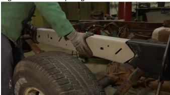
Remove any potential fire hazards from the work area. Tac weld the part to the frame. Following proper welding procedures, begin welding the part.
