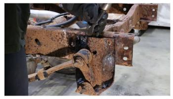
Begin cleaning the area free of rust and debris, revealing bare metal.
