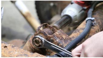
Begin removing your rear spring hanger by cutting off and prying out its rivets.
