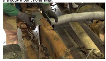
Assemble the crossmember by inserting the pipe through the frame and its bounding plates. Ensure the rotation and placement of the tube and shock mount matches factory orientation.
