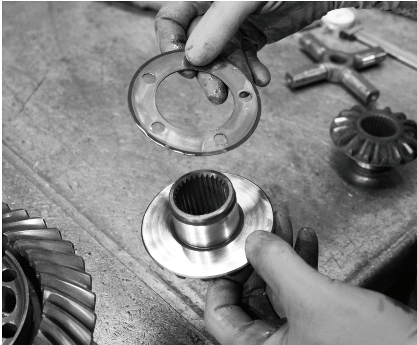
Figure 1 - MUST REMOVE thrust washers
