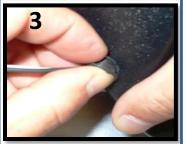
Feed the spade terminals through the 7/16" hole on back of each pod and push grommet into hole.
