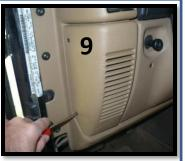
Remove the speaker covers from your TJ's dash with a Phillips screwdriver, 2 screws per side.
