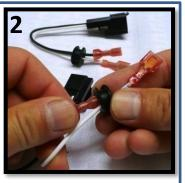
Push grommet over each pair of plugs starting with the large spade first. It's a tight fit, but it minimizes hole size.
